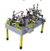
Bluco's modular fixturing system for welding features 3-D tables and a complete family of modular elements that can be assembled quickly and accurately to fixture just about any size and type of part. Prototype and production versions of this go cart frame are built using a standard set of modular tooling components. Applications include pipes, sheetmetal, roll-over fixtures and many more.
