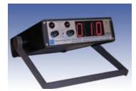
The new ARGWELD® Critical Weld Purge Monitor measures residual oxygen levels down to 0.001% (10 parts per million) and is specifically designed for applications involving reactive materials such as titanium and duplex. The unit has an 02 level alarm, comes with a new low-maintenance sensor with a five year life expectancy and an automatic pump. An optional software package is available to store and print results for quality control purposes.
