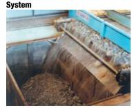
Rapid Clean permits the automatic extraction of slag and scraps produced during sheet metal cutting. Steel brushes and blades slide across a sheet metal plate, being driven by a motor-reducer and by resistant chains. The latter are held by special slide bars located on the side of the suction channels. The main advantage is the avoidance of the constant cleaning of the scrap collecting boxes under the cutting machine.
