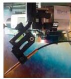
PTR introduces its latest accessory for EB welding systems, a 3-Axis CNC Controlled Wire Feeder. This proprietary wire feeding and locating system adds another level of capability to PTR EB Welders. Wire position can be moved in 3 axes and the motion control is integrated directly into the system's CNC. Uses include build ups for EBAM (Electron Beam Additive Manufacturing), adding filler materials, weld repairs and others.
