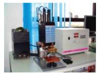
Will-Best introduces its spot welder WBT-Q03H+DP-875 precision weld power supplies. The supplies are good for 18650 and 26650 power battery pack welding, and could weld 0.1—0.5mm battery tabs and 1.0mm metal stripes. In addition, they are good at cycle welding (weld over 4000pcs/day), have pneumatic welding style and ensure the consistency of welding and have firm welding point, avoid loose welding; easy operation; low breakdown rate and quick service.
