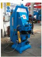
The new and improved SERTOM C-25 Plate Beveling machine brings robust power to your fabricating shop. With completely hydraulic operation the C-25 will provide years of trouble free beveling operations. The C-25 also provides the ability to invert the unit for "bottom side" plate beveling without the need to "flip" the plate manually. The C-25 is fast, rigid, has plate thickness capacity of 65mm and utilizes "off the shelf" cutters.
