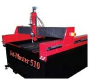
Advance Cutting Systems is pleased to introduce the new JetMaster WaterJet Cutting Machine. Driven by Hypertherm's Edge Ti Color Graphic Control, and using an H2O, 60,000 PSI Pump, the JetMaster is priced to meet even the tightest budget. Key features include the ability to raise and lower the water height, and the recirculating water cooler on the H2O Pump saves on water consumption.
