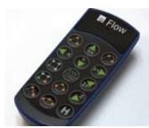
FlowTeach™ is designed to quickly digitize patterns, templates or parts into FlowMaster® software. This easy to use, intuitive system is available for all Flow Mach series waterjets and can be retrofitted onto most legacy Flow systems. It allows the operator to jog the Flow machine tool around the periphery of the part or template, selecting points and thereby recreating the geometry within the FlowMaster control.
