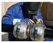
The Hot Coils® new pipe preheating technology gives you a heating crew at your command. Just snap on the quick heating coils and plug into any 110 volt, 15 amp. power source. No special set-up labour, no waiting for high cost specialized equipment or heating services, and no highly flammable gasses or high voltage cable runs to deal with.
