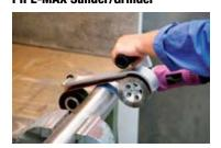
PIPE-MAX sander/grinder efficiently deburrs, grinds and polishes closed and open pipe constructions from 3/8" to 12" diameter. Belt speed adjustments from 33 to 100 ft./sec. allow rough grinding or polishing on stainless steel, aluminum and steel. Balanced, adjustable handles for right or left-handed use. Soft, elastic return roller provides flexibility to adapt to every pipe contour. Grinding action removes spot welds and deep scratches from flat surfaces.
