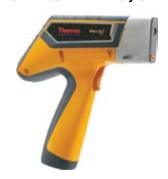
The new lightweight, yet ruggedly built Thermo Scientific Niton XL2 GOLDD analyzer delivers high performance in a value package. With a standard analysis range of more than 25 elements, it brings exceptional accuracy, precision, and ease of use with its fast analysis, high throughput, and the added ability to measure light elements (Mg-S) without helium purge or vacuum. From turn on to trigger pull to confident results in seconds.
