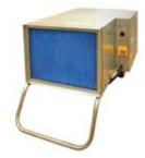
Fostoria's new "Hot Room Heater" Series can quickly and efficiently heat rooms up to 150 degrees F., to bake, cure, dehydrate, or in general heat products or coatings requiring heat in a non-hazardous environment. Units can be permanently mounted or portable, and with the option of the inlet and outlet air ducted to and from the room. Variety of Kw at all industrial voltages.
