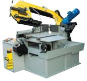
The FMB Pegasus DS offers semi-automatic operation of the cutting cycle, complete with hydraulic clamping, positive hydraulic cutting pressure and auto return after the cutting cycle. This model is capable of mitering 60 degrees to the left AND 60 degrees to the right! It also comes standard with a digital display of the cutting angle and a 1-1/4" wide band. The cutting capacity is 20".
