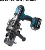
Hougen Manufacturing introduces the new 18V Cordless Hole Puncher. The battery powered model 76000 can punch holes up to 19/32" in diameter through 15/64" steel. The unit can punch holes in flat bar, angle iron and channel, weighs just 16.5 lbs and produces 8.5 tons of pressure. The Lithium-ion battery can be charged in just 22 minutes and has the capability to punch up to 150 holes.
