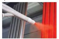
The Prodigy® HDLV (high-density powder, low-velocity air) spray system incorporates a high-capacity transfer pump, delivery pump and guns, offering an integrated solution for precision dispensing, exceptional repeatability and improved process control. Prodigy HDLV systems move more powder with less air to create a softer spray pattern, higher first-pass transfer efficiency, faster coating and better part coverage.
