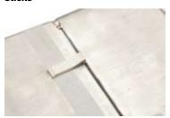
Made from Aquasol® Water Soluble Composite Board, Solu-Shim™ Alignment Sticks maintain a precise gap between pipes, plates and even flanges. Features include: required minimum gap for plate/pipe projects as required by AWS codes D1.1 thru D1.6; and API 1101 pipe codes; easily and quickly installed; effortlessly removed with introduction of water; and eliminates the need for costly post-weld grinding.
