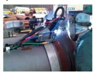
The Pipe Kat from Gullco is a complete welding system with integrated wire feeder for orbital welding and field pipeline use. Works on pipes from 10" outside diameter and up to flat. The carriage incorporates a 40 IPM wire feeder, remote pendant control, programmable control box, oscillator head and high speed carriage to increase efficiency and arc on time in field pipeline welding.
