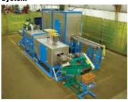
The system is used for coating small parts for cosmetic appearance and corrosion resistance. Components include: convection preheat oven, automatic feed fluidized-bed coating system, transfer conveyor, and automatic weighing scale. The infrared re-flow oven makes the system extremely energy efficient.
