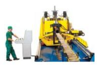
With a new OLIMPIA80 patent, this machine has been designed for the in-line cutting of large dimension tubes, in round, square and rectangular shapes, with speeds up to 85 m/min. The innovative system with parallel movement of blades reduces the cutting cycle time andthe set up of the blades easier.
