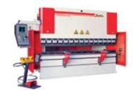
The new Baykal APHS press brake features a new high speed hydraulic package that is standard on all APHS machines. The larger open height and deeper throat allow for more parts to be formed. The machine is equipped with the standard front support arms on linear guides, Baykal CNC crowning, a 4 axis servo driven back gauge, side and rear interlocked safety, and the Delem 66W color graphic controller.
