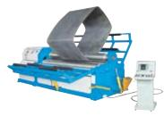
Knuth Machine Tools offers the RBM series CNC plate roll bending machines for bending elliptical and conical forms, pre-bending and bending in one operating step. Equipped with hardened rollers and a rigid construction, the RBM is available with CNC or NC Teach-In controls to handle infinitely variable turning speeds.
