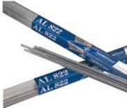
The new AL-822 Handy One® aluminum alloy is suitable for brazing of aluminum-to-aluminum and aluminum-to-copper. AL-822 Aluminum Handy One, with its lower melt point, makes it easier to join components such as aluminum condensers and evaporators, and other aluminum base metals when compared to other aluminum braze alloys. Easy to use, AL-822 includes a noncorrosive flux eliminating the need for a separate flux.
