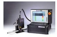
Designed for the tube and pipe industry, the WI2000p detects quality issues related to the welding process.
