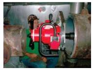
E.H. Wachs introduces an I.D. mount end prep machine tool designed to bevel, compound bevel, J prep, face and counterbore pipe, fittings and valves. Speed Prep feeds simultaneously in the axial and radial planes, machines bevel or compound bevel without templates, incline tool slides or work stoppage. The EP 424 can form a tool 4" - 16" to Schedule 160, single point 4" - 24" up to 6.5" wall thickness.
