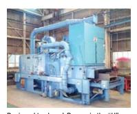
Designed to clean I-Beams in the "H" position, the SCRA-12H provides descaling of structural shapes with down stream operations in mind. Superior cleaning through improved wheel angles and a patent pending abrasive removal system make this machine a must for today's Structural Fabrication Industry.
