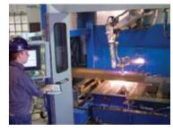
PythonX Structural Fabrication System does the work of a Beam Drill Line, Band Saw, Coping Machine, Angle Fabrication Machine and a plate/bar line. By doing all structural fabrication on one machine, PythonX users produce at the lowest cost because they eliminat material handling between operations and automate structural fabrication of bolt holes, copes, cut to length, labeling, weld prep bevels, stair stringers and beam splitting. Structural Steel Fabrication reinvented.
