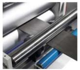
PowerFeed coil feed is designed to meet the demands of servo presses. It boasts a system accuracy of  $\pm$  0.05 mm achievable over long periods. The roller coating ensures that high accelerations are effectively transferred to the material. Available in three model ranges, "Light" for up to 100 kilograms of movable mass, "Medium" for up to 180 kilograms and "Heavy" for up to 300 kilograms of moveable mass.
