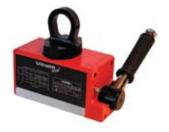
The Ultralift Plus<sup>™</sup> is a safe and only permanently magnetic lifting magnet equipped with a patented safety shim which allows pre-testing of any load to ensure a 3:1 safely factor. The unique lifting eye mechanism (patent pending) ensures that the lifting magnet cannot be switched off when holding a load. The Ultralift Plus is easy to use and won't mark the finish of the load.
