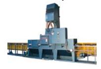
The Viking SR-6 Pipe and Rod Blaster can remove rust or enamel from a wide variety of materials, from fractional diameter up to 6-inch pipe to an SSPC-6 surface finish on a continuous flow basis. The skew roll conveyor system handles the pipe/rod through the blast chamber on precision cast chrome rollers providing maximum efficiency and cleaning throughput of 5-30 feet per minute.
