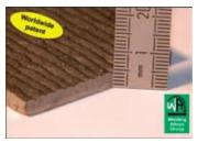
Welding Alloys Hardlite<sup>™</sup> features an extremely refined micro-structure with high volume of chromium carbides alloying an ultra high wear resistance. 68 HRC is achieved through the company's unique patented process. Applications include cones, endless screws, tubes, armoring app., crushers, classifiers, fans in steelmaking, cement ind., quarries, agriculture, and thermal power stations.
