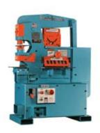
The 50514-CM, five-station, 50-ton ironworker's standard features include: 50-ton punch station, 4" angle shear, 14" flat bar shear , built-in rectangle notcher capable of notching 2-1/2" x 3" x 5/16", and a fifth station, located next to the angle shear, which allows an optional pipe notcher to be mounted without removing the angle shear.
