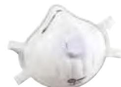
a flame-retardant outer layer that provides crucial protection for welding operators in environments where sparks or spatter could come in contact with the mask. The filter media offers 95 percent filtration of airborne particles, including hexavalent chromium, manganese and other weld fumes. An integrated valve eases breathing for the user.
