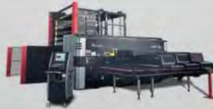
LC 2515 C1 AJ Punch/Fiber Laser Combination with ASR Automation
